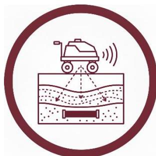
At Geopin, we offer Ground Penetrating Radar (GPR) surveys, a critical non-destructive method that uses radar pulses to image the subsurface. We detect and map features and objects beneath the ground, such as **underground utilities (pipes/cables), rebar in concrete, and geological anomalies**. This technique is essential for preventing damage during excavation, assessing infrastructure condition, and safely providing an accurate 'x-ray' of what lies below.
